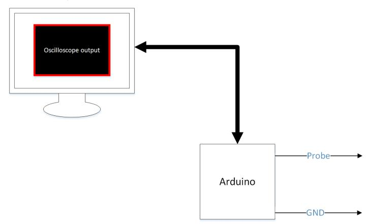
The Arduino board contains a 6 channel, 10-bit analog to digital converter. This means that it will map input voltages between 0 and 5 volts into integer values between 0 and 1023. This yields a resolution between readings of: 5 volts / 1024 units or, .0049 volts (4.9 mV) per unit.
