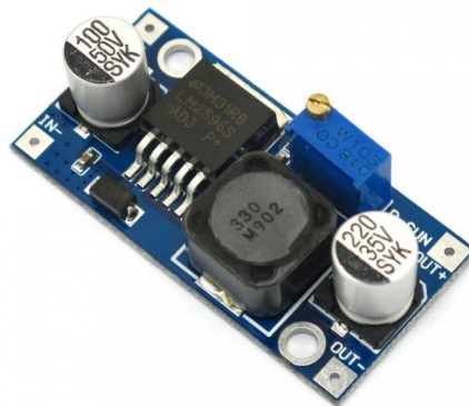
Figure 4-5. LM2596S Step down converter
