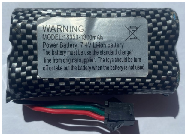
Figure 5-10. 7.4V Li-Ion Battery Pack
